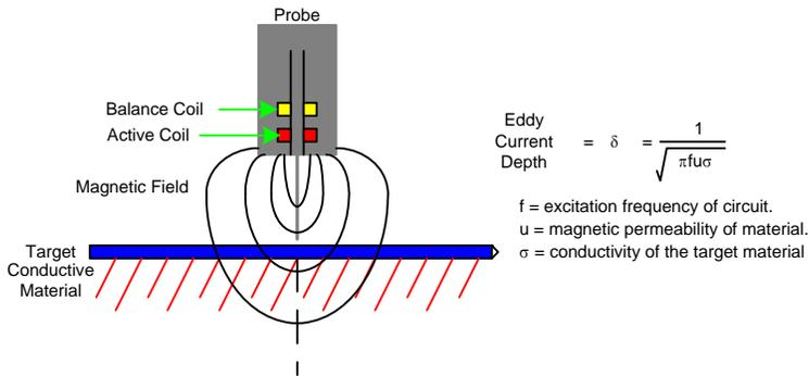
The test system places an exciting coil that generates a high frequency magnetic field close to (but not touching) the target specimen to create the eddy currents. These induced currents produce a secondary magnetic field. Measuring the resulting field composed of the primary and secondary fields, the sensor receives the target specimen characteristics: electrical conductivity, thickness, shape and the sensor-target distance (“lift-off”).
